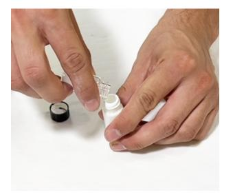
Pour Paint (A) & Texture (B) into Catalyst (C). Close Catalyst bottle (C) and shake for one minute to mix contents.
